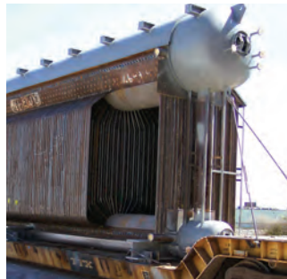
250,000 lb/hr 725 psig superheated boiler system.
